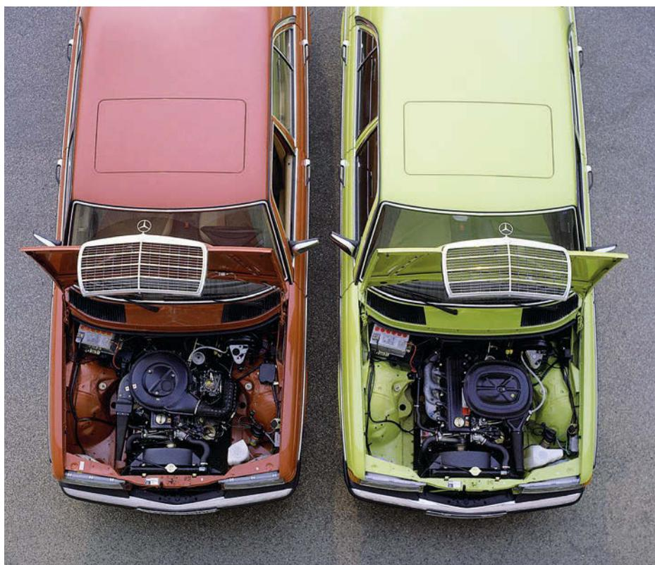
The 2.0 unit as fitted the the W123 Mercedes 200 had an 87 mm bore and a crank stroke of 83.6 mm to give a capacity of 1988 cc. The unit featured a double roller (duplex) timing chain, forged steel crankshaft and the promise of a long life. Carburation was by a single Stromberg CDT 175 carburettor.
